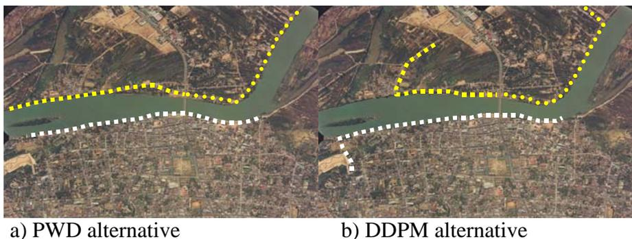
Fig. 5 Proposed Alignment of Retaining Wall by PWD and DDPM.
