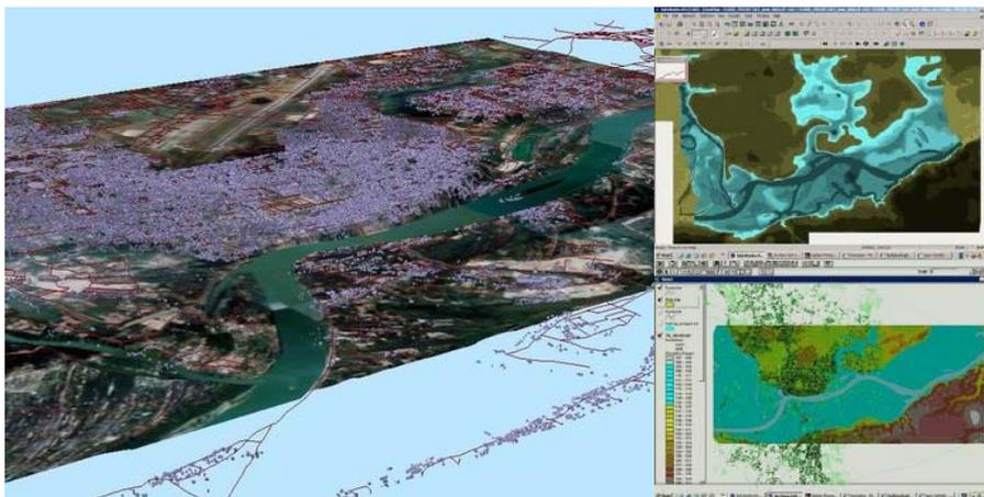
Fig. 7 Computer Simulation Output: Boundary of Flooding at Water Level +116 MSL.
